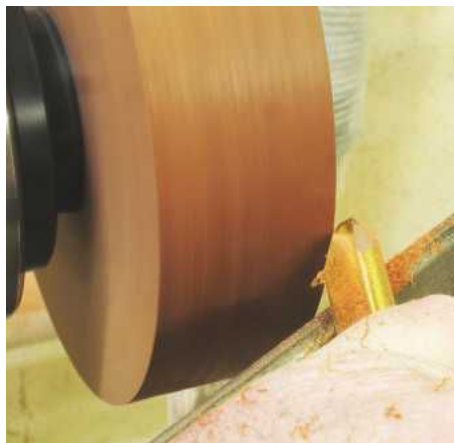
▲ Pic.8 You can take the arris off the edge either with the tool or, if you are not confident doing that, use a piece of abrasive. To avoid dig in if using a tool keep the flute pointing at 3 and 9 o'clock
